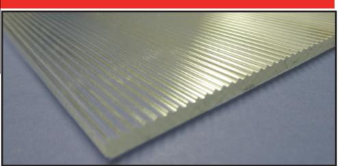
The P25 Clear Linear Prism is distinctive due to the design of the prism across the width of the sheet. The linear prisms are finished with a textured surface to help eliminate the lamp image and increase the sheets light transmission consistency.
