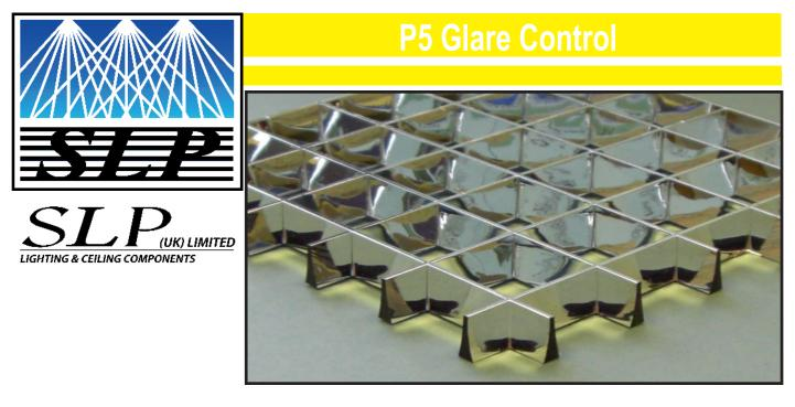
The P5 Louvre is the least expensive product in the Para-square range with the shallowest cell configuration. The P5 is the low brightness louvre of choice when energy budgeting and controlled luminance are critical. The flat backed 20x20x9mm cells enable the louvre to maintain 99% of its light distribution in the 0-60 zone.
