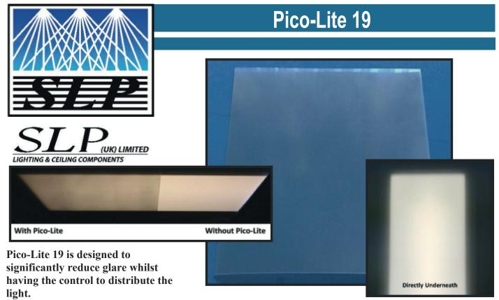
Arguably the best <UGR19 material available, Pico-Lite 19 has been manufactured with glare reduction at the forefront of its design. Available as a film or solid sheet, Pico-Lite 19 is a unique product boasting high light transmission whilst suppressing high angle light above 65 degrees. Independent photometric tests show <UGR19 results under almost all circumstances due to the optimal prism design and size and can reach this with an output of up to 5000 lumens.
