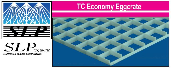
The TC Economy Eggcrate Louvre is designed to give maximum lighting output through the 15 x 15 x 8 mm cell configuration. This louvre is injection moulded on the most modern computer controlled system and each individual louvre is coated with an anti-static fluid to prevent the airborne dirt and dust from sticking to the cell walls during installation.
